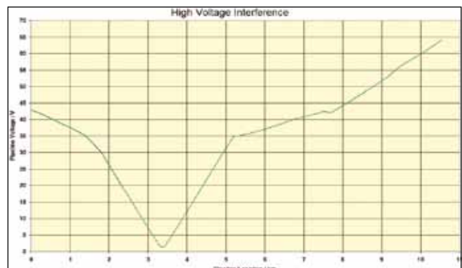
Calculation results caused by overhead line operating currents with earthing measures ( U_{max} < 65 V according to German Standard)
