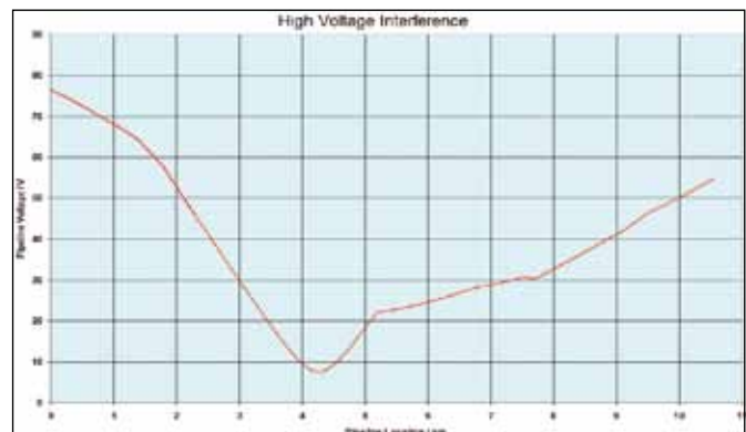
Calculation results caused by overhead line operating currents without any earthing measures
