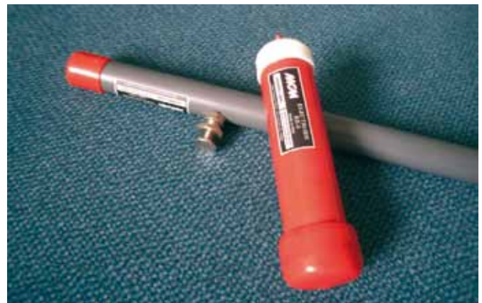
Reference Electrode Cu/CuSO 4 for use in soil and (with submersible adapter) for use in water Model: MILLER RE-5
