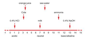
The pH scale is logarithmic. A difference of one pH unit represents a tenfold, or ten times increase or reduction of hydrogen ion activity in the solution. This explains how a solution's aggressiveness increases with the distance from the neutral point.
