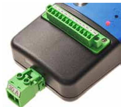
4 DC and 4 AC Inputs 30A relay for switching rectifier regulation
