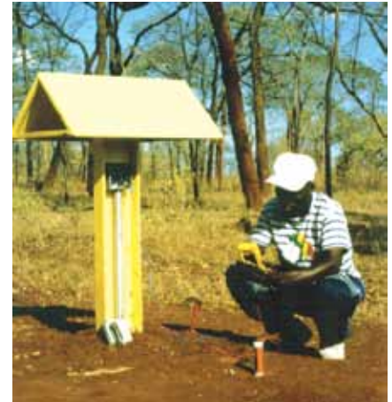
Type - CR - For checking interference between the protected pipeline and other pipelines or structures as well as pipe-to-soil potential measurements
